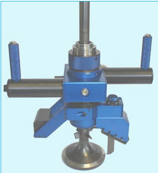
Refacing Valve Face
