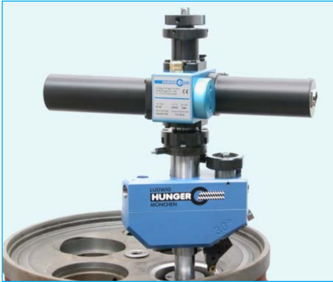
Refacing Valve Seat
