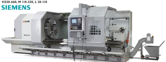
The XYZ XL and Oil Country Lathes are heavy-duty machines built to handle the toughest of work for either chucking or between centre applications using the massive tailstock assembly. The solid ribbed cast construction with wide vee and flat bed ways offer excellent stability and rigidity. The powerful spindles sit in a headstock built using the highest quality gears and bearings.
