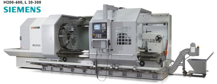
The XYZ XL and Oil Country Lathes are heavy-duty machines built to handle the toughest of work for either chucking or between centre applications using the massive tailstock assembly. The solid ribbed cast construction with wide vee and flat bed ways offer excellent stability and rigidity. The powerful spindles sit in a headstock built using the highest quality gears and bearings.
