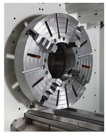
The XYZ Oil Country and XL Lathe range feature a one-piece bed and base casting.
